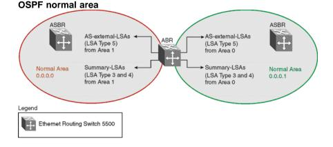
The Nortel Ethernet Routing Switch 5500 Series automatically becomes an ABR when more than one area is configured for it and each area has at least one operational interface. To designate a router as an ASBR, use the **as-boundary-router enable** command.
